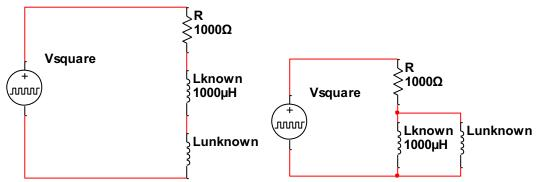
In this section, you are provided with a known inductor (1000  $\mu$ H) in series with an unknown inductor. Then, the known inductor (1000  $\mu$ H) will be in parallel with an unknown inductor. After we solve for the total L, we can find the unknown inductor from the parallel or series equation. In series, the inductors are related by the equation:  $L_{eq} = L_1 + L_2 + ... + L_n$ . In parallel, the inductors are related by  $1/L_{eq} = 1/L_1 + 1/L_2 + ... + 1/L_n$ .
